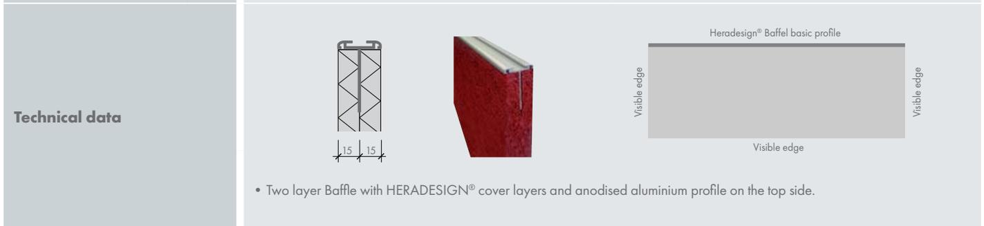
**Fire reaction** Euroclass B-s1,d0 and A2-s1,d0 according EN 13501-1
